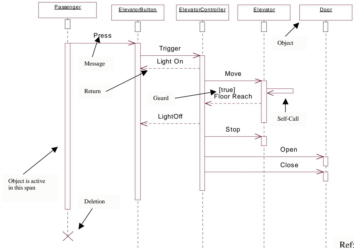
A **Lifeline** represents the duration during which an object is alive and interacting with other objects in the system. It is represented by dashed lines. The long, thin boxes on the dashed lines represent method activations and they indicate that a process is being performed by the target object to fulfill a message. A **Self-call** occurs when an object sends a message to itself. In
