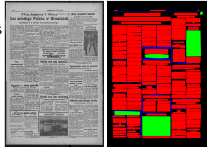
Figure 4. Example of image (left) and ground-truth (right) from ENP dataset. In the ground-truth, each color represents the following components: (1) black: background, (2) red: text, (3) green: figure, (4) blue: line-separator, and (5) yellow: table.
